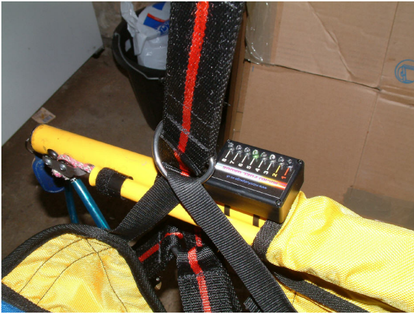
The display unit. The different LEDs light up as the fuel level drops until the last red light tells you it'll soon be time to land.
