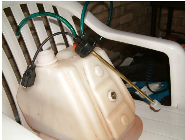
The float slides down the bar as the fuel level drops, triggering the different LEDs in the display unit.
