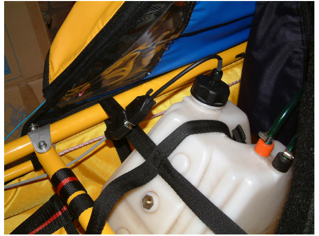
The display unit connects to the sender in the tank. It's only switched on if it's plugged in.
